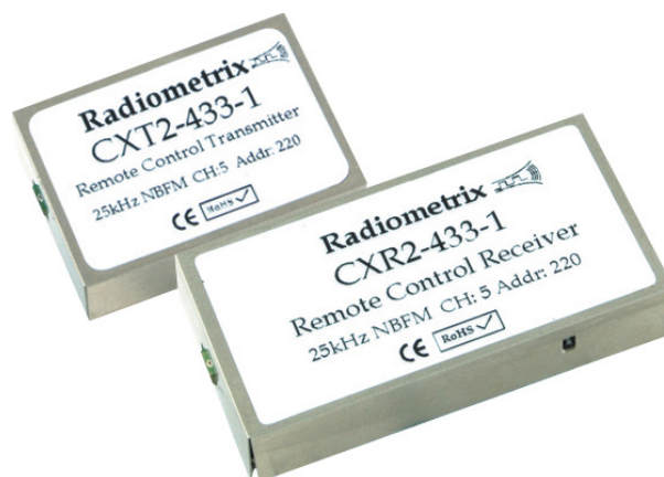
Figure 1: CXT2 transmitter and CXR2 receiver
