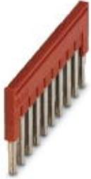
Plug-in bridge, pitch: 5.2 mm, length: 22.7 mm, width: 50.6 mm, number of positions: 10, color: red
