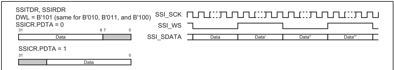
Figure 32A.30 Bit Alignment in 18-/20-/22-/24-Bit Stereo Format
