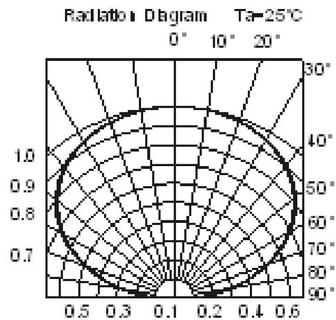
Typical Electro-Optical Characteristics Curves
