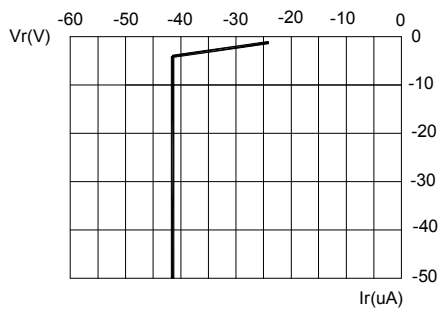
FIG.3 RED & AMBER REVERSE CURRENT VS. REVERSE VOLTAGE.
