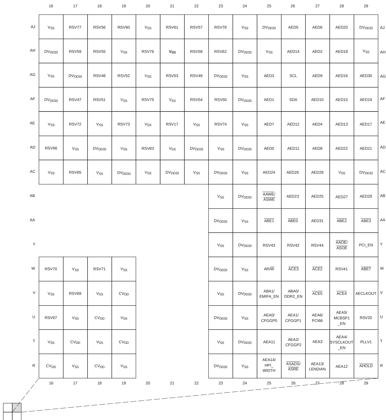
Figure 2-3. C6454 Pin Map (Bottom View) [Quadrant B]
