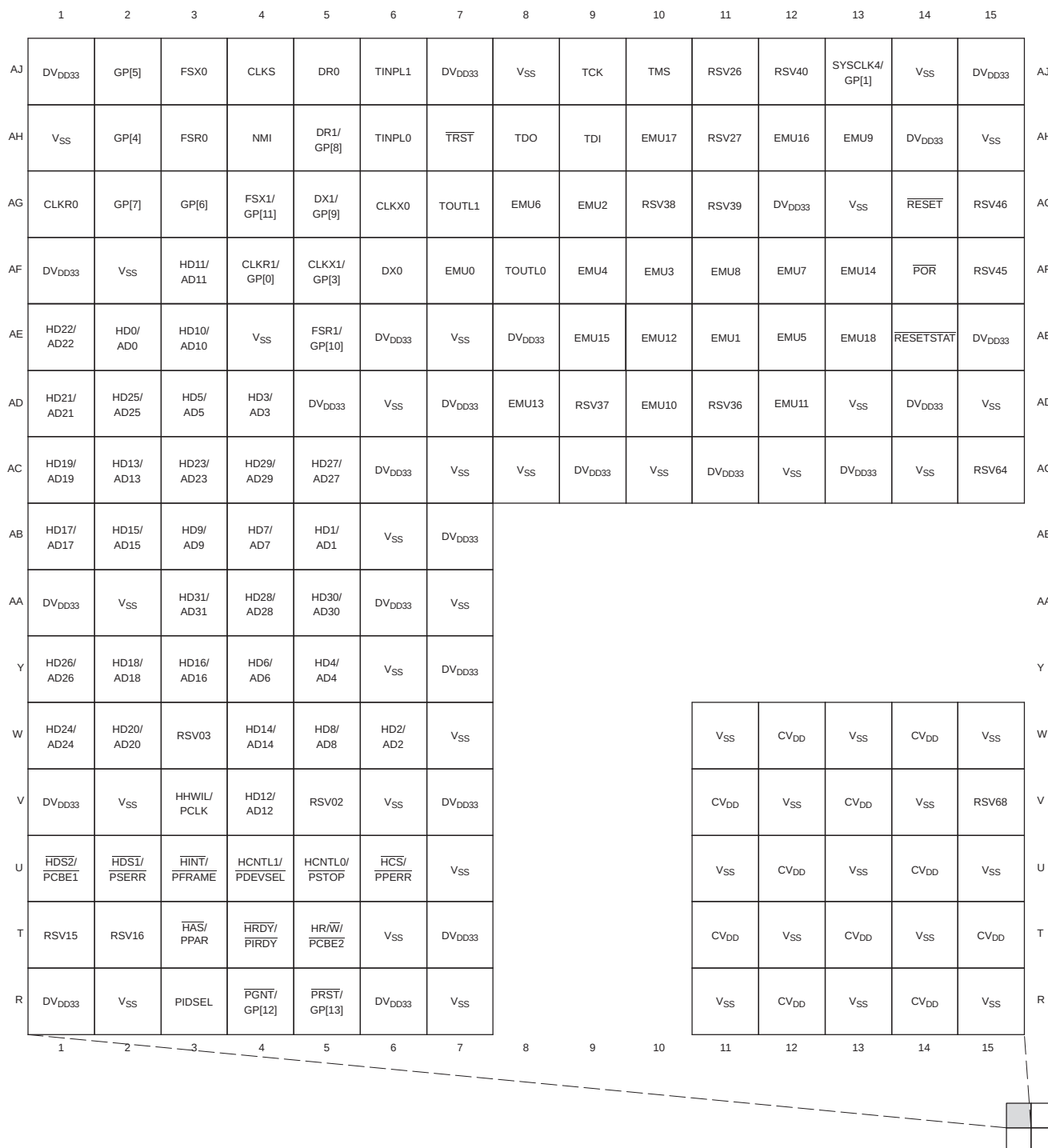
Figure 2-2. C6454 Pin Map (Bottom View) [Quadrant A]
