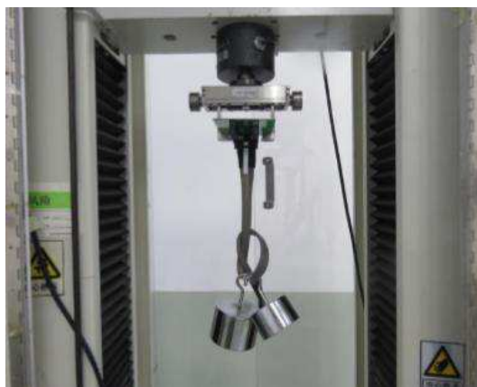
Figure 2 – Latch retention Test Setup
