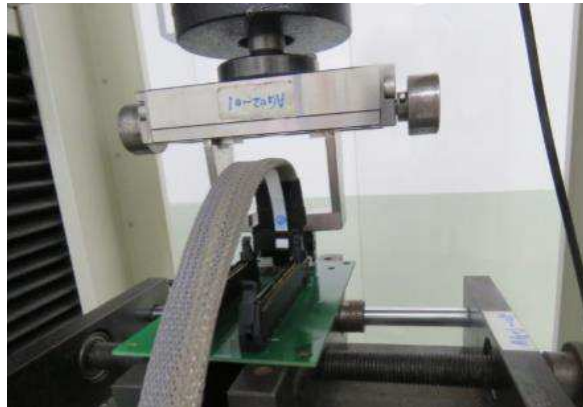
Figure 6 – Mating Force Test Setup
