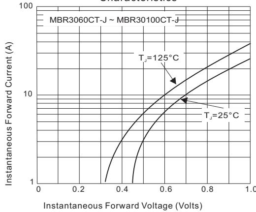
Fig. 3C - Instantaneous Forward Characteristics
