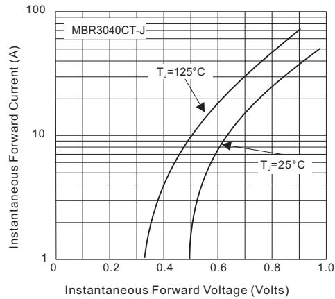
Fig. 3B - Instantaneous Forward Characteristics
