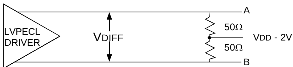
Test Circuit for LVPECL Output Characteristics
