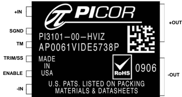
Figure 2 Picor PI3101-00-HVIZ Pin Out
