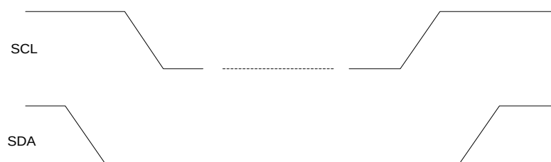
Figure 34: I 2 C START and STOP Conditions
