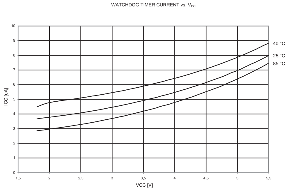
Figure 21-16. Watchdog Timer Current vs. V_{CC}
