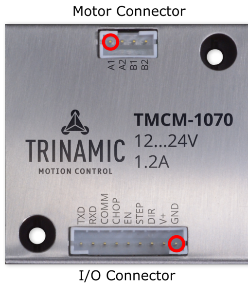
Figure 7: TMCM-1070 connectors (pin 1 highlighted in red)
