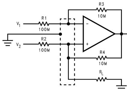
**Figure 23. Howland Current Pump Guard Ring Connections**
