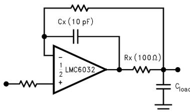
Figure 17. Rx, Cx Improve Capacitive Load Tolerance
