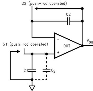
**Figure 25. Simple Input Bias Current Test Circuit**
