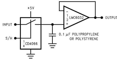
Figure 28. Low-Leakage Sample-and-Hold
