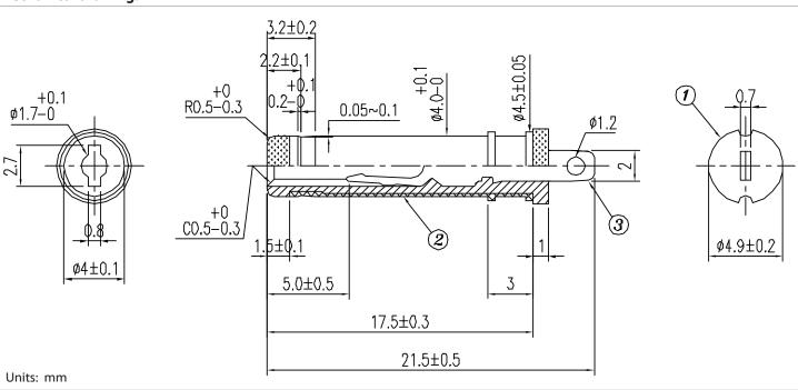
tolerance X:  $\pm 0.5 \, \text{mm}$  .X:  $\pm 0.3 \, \text{mm}$  .XX:  $\pm 0.05 \, \text{mm}$  applicable unless otherwise indicated in specification or on drawings
