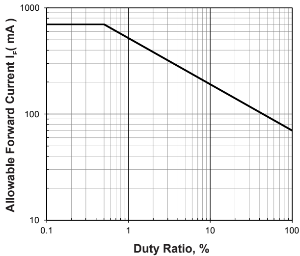
Allowable Forward Current Vs Duty Ratio
