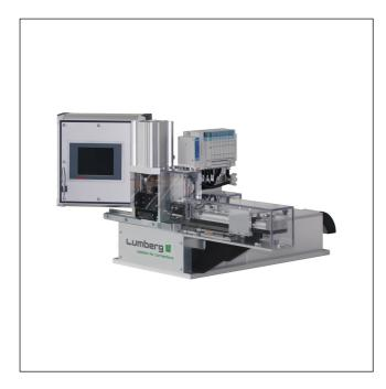
Semiautomatic harnessing machine for termination of RAST 2.5 connectors in insulation displacement technology, small base machine, limited upgrading possible
