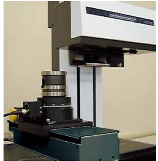
Example of Y-axis CNC table (100 mm) and \theta -axis CNC table (horizontal) combination
