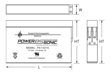
HT: 3.52 (89) **L**: 5.91 (150) **W**: 0.80 (20) H: 3.52 (89) Tolerances are +/- 0.04 in. (+/- 1mm) and +/- 0.08 in. (+/- 2mm) for height dimensions. All data subject to change without notice.
