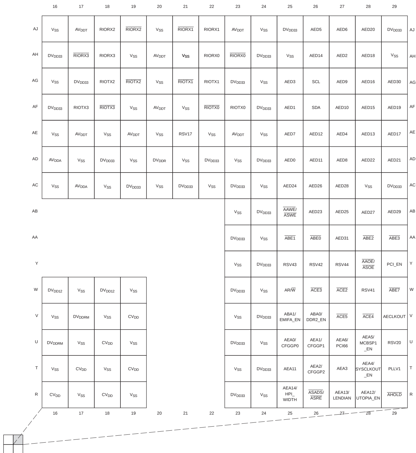
Figure 2-3. C6455 Pin Map (Bottom View) [Quadrant B]
