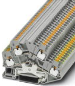
Protective conductor double-level terminal block, Cross section: 0.14 mm 2 - 4 mm 2 , AWG: 26 - 12, Connection type: Push-in connection, Width: 5.2 mm, Color: gray, Mounting type: NS 35/7,5, NS 35/15
