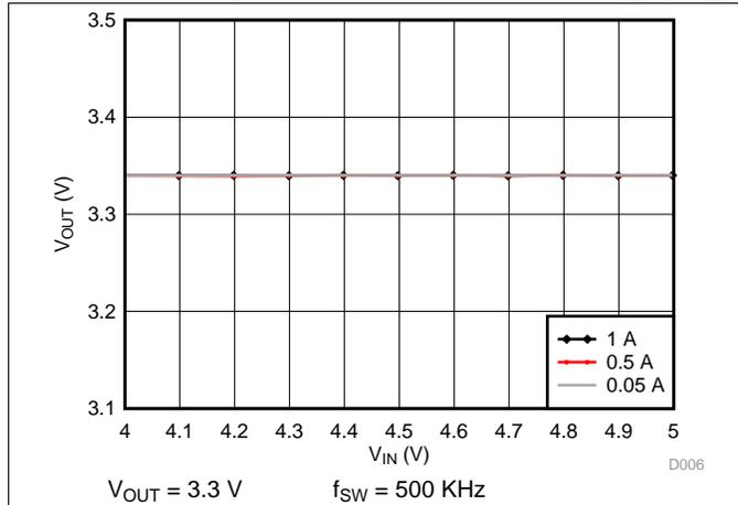
Figure 7. Dropout Curve
