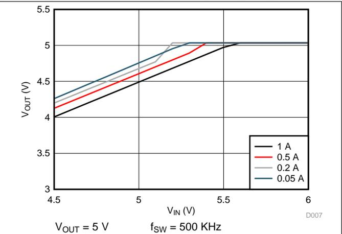
Figure 8. Dropout Curve
