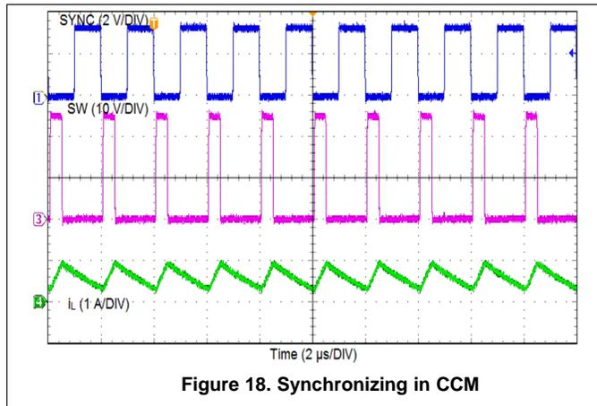
Figure 18. Synchronizing in CCM
