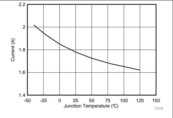
Figure 10. High-Side Current Limit vs Junction Temperature
