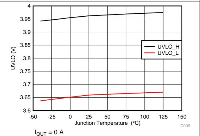
Figure 12. UVLO Threshold
