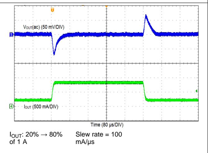
Unless otherwise specified the following conditions apply:  $V_{IN} = 24\text{ V}$ ,  $f_{SW} = 700\text{ KHz}$ ,  $L = 15\text{ }\mu\text{H}$ ,  $C_{OUT} = 47\text{ }\mu\text{F}$ ,  $T_A = 25\text{ }^\circ\text{C}$ .
