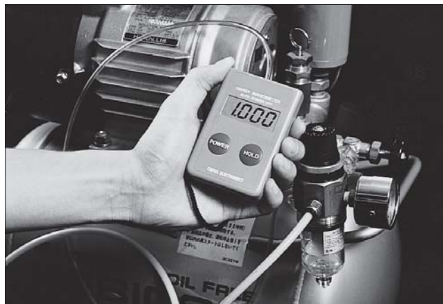
▲ Measurement of source pressure from a compressor.
