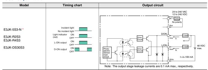
Note: Connect the brown cable to any polarity and the blue cable to the power supply because there is no polarity on the Emitter side.
