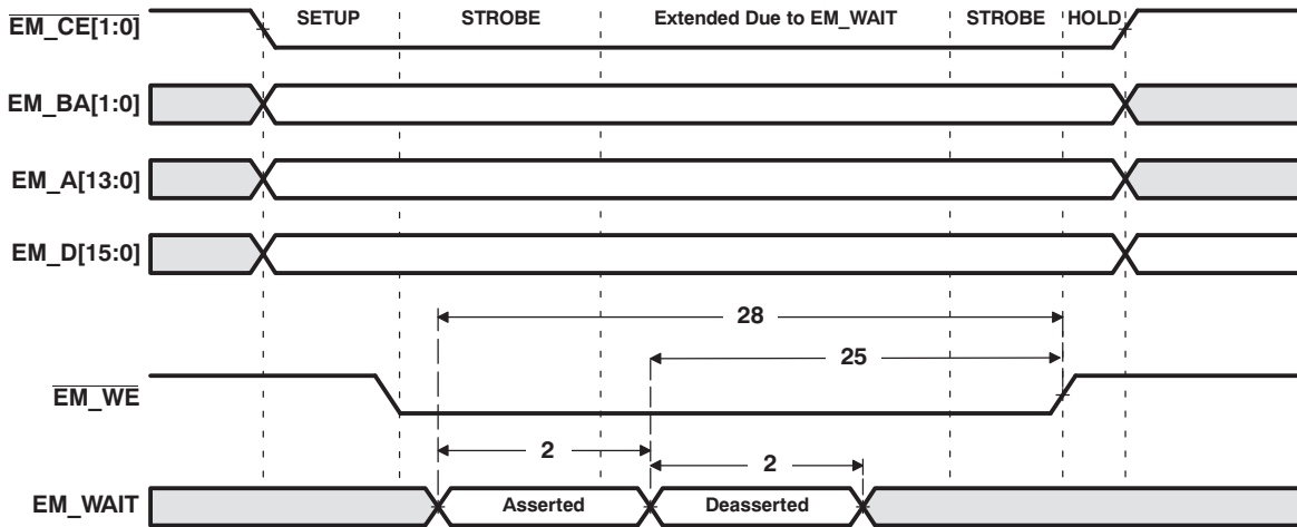
Figure 5-17. EM_WAIT Write Timing Requirements
