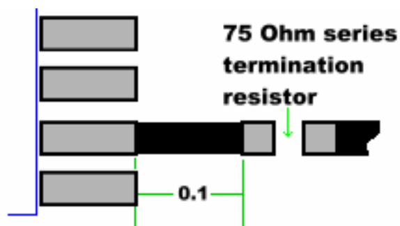
Figure 3. Proper Termination Resistor Placement
