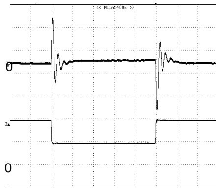
Figure 9: Output voltage response to step-change in load current (75%-50%-75% of I_{o, max} ; di/dt = 1.0A/\mu s ). Load cap: 100 \mu F tantalum capacitor and 1 \mu F ceramic capacitor. Top Trace: V_{out} (100mV/div, 200us/div), Bottom Trace: I_{out} (10A/div). Scope measurement should be made using a BNC cable (length shorter than 20 inches). Position the load between 51 mm to 76 mm (2 inches to 3 inches) from the module
