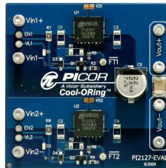
Figure 1: PI2127-EVAL1 Evaluation Board (1.8" x 1.8")
