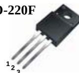
1.Gate 2. Drain 3. Source
