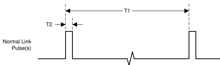
图 7-13. Normal Link Pulse(s) Timing
