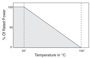
Case Temperature is measured on the metal mounting tab against the molded body
