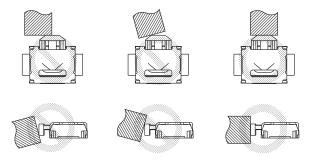
Do not operate the plunger from the side. Doing so may deform or damage the Switch.
