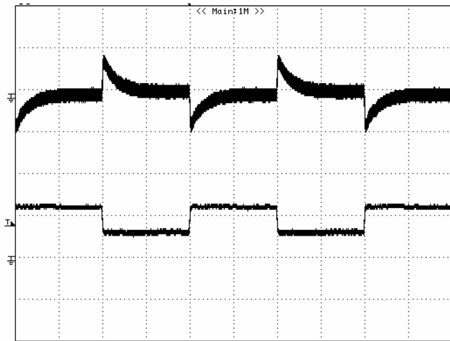
Figure 6: Output voltage response to step-change in load current (50%-25%-50% of I_o , max; di/dt = 0.1A/\mu s ). Load cap: 10 \mu F , tantalum capacitor and 1 \mu F ceramic capacitor. Top Trace: Vout (200mV/div, 500us/div), Bottom Trace: I out (2A/div). Scope measurement should be made using a BNC cable (length shorter than 20 inches). Position the load between 51 mm to 76 mm (2 inches to 3 inches) from the module
