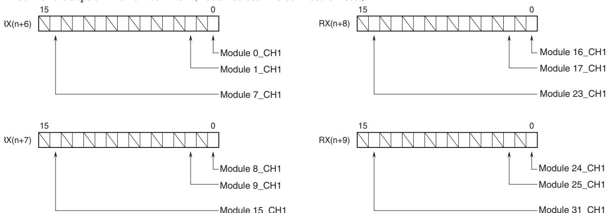
Note: In Data Allocation mode “1,” CH2 is invalid, and its all bits turn to “0.”
