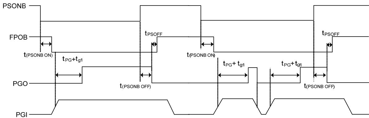
2)  $V_{33}, V_5, V_{12A}, V_{12B}$  (UNDER-VOLTAGE) or  $I_{S33}, I_S5, I_{S12AB}$  (OVER-CURRENT):
