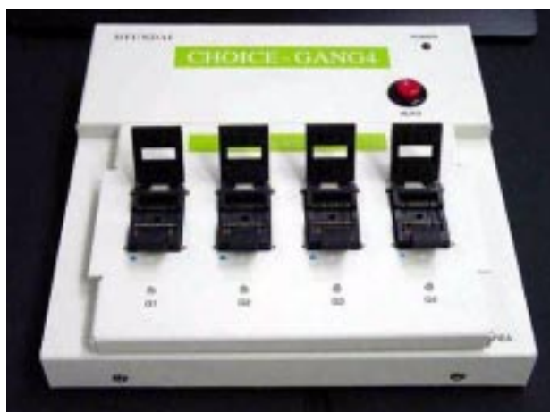
Figure 1-3 OTP Gang Programmer CHOICE-GANG4 TM
