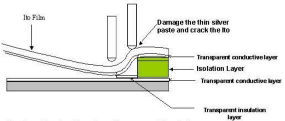
Pen input load on the edge of transparent insulation area might damage the ITO of ITO Pet- Film and reduce the durability of touch panel
