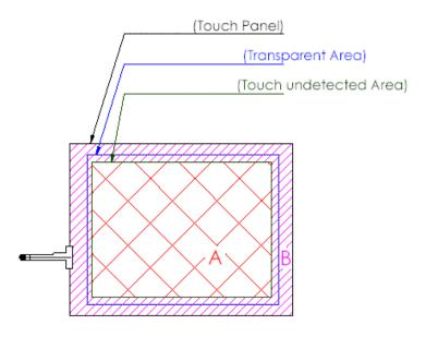
A area: Without any defect point effect on normal operation.
