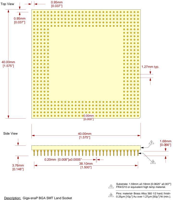
520 position BGA surface mount land pattern to terminal pins (1.27mm [0.050"] centers, 31x31 array)
