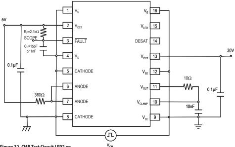
Figure 32. CMR Test Circuit LED2 on
