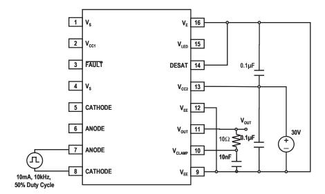
Figure 29.  $t_{PLH}$ ,  $t_{PHL}$ ,  $t_{f}$ ,  $t_{r}$ , test circuit
