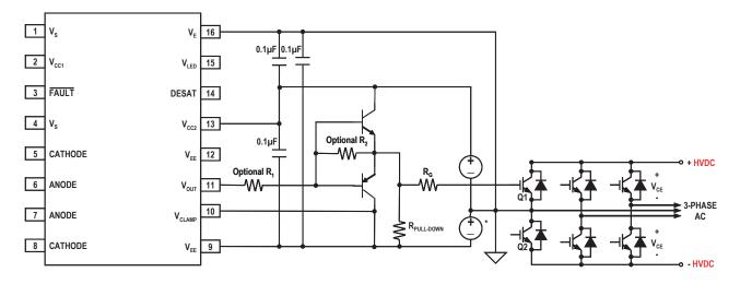
Figure 40. IGBT drive with negative gate drive, external booster and desaturation detection (V<sub>CLAMP</sub> should be connected to V<sub>EE</sub> when it is not used) VCLAMP is used as secondary gate discharge path. \* indicates component required for negative gate drive topology
