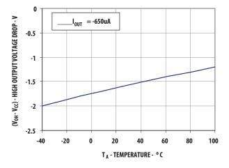
Figure 4. V<sub>OH</sub> vs. temperature
