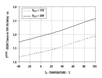
Figure 18. DESAT sense to 10% VOUT delay vs. temperature
