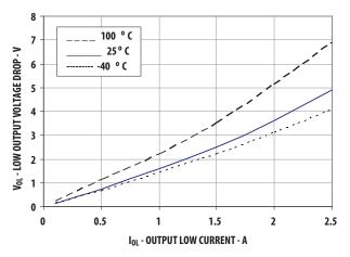
Figure 7. V<sub>OL</sub> vs. I<sub>OL</sub>
