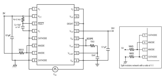
Figure 34. CMR Test Circuit LED1 on
