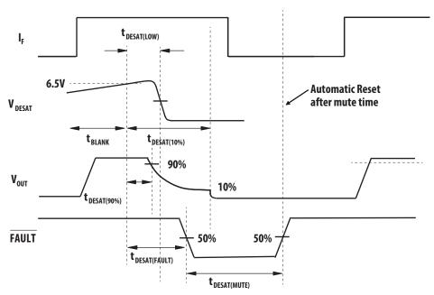
Figure 37. Fault Timing diagram (ACPL-333J)
