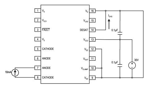
Figure 27. I<sub>CHG</sub> Pulsed test circuit
