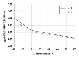
Figure 9. I<sub>CC2</sub> vs. temperature
