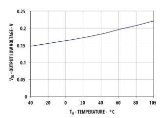
Figure 5. V<sub>OL</sub> vs. temperature
