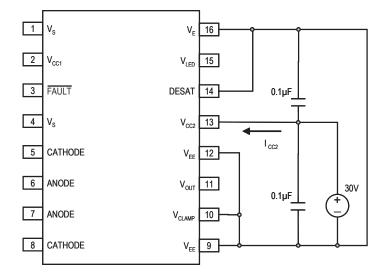
Figure 26.  $I_{\text{CC2L}}$  test circuit
