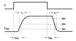
Figure 1. VOUT propagation delay waveforms
