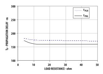
Figure 15. Propagation delay vs. load resistance
