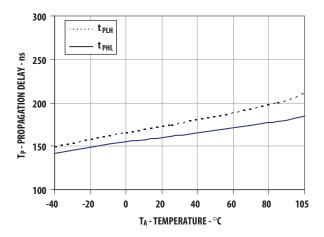
Figure 13. Propagation delay vs. temperature
