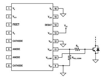
Figure 38. Output pull-down resistor.
