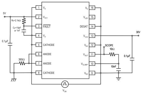
Figure 33. CMR Test circuit LED1 off
