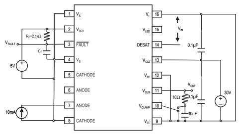
Figure 30.  $t_{DESAT}$  fault test circuit
