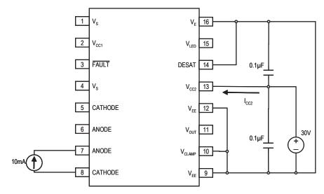
Figure 25. l<sub>CC2H</sub> test circuit
