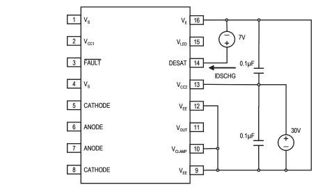
Figure 28.  $I_{DSCHG}$  test circuit
