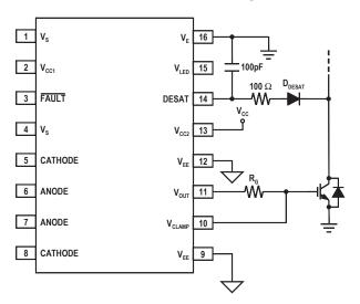
Figure 39. DESAT pin protection.
