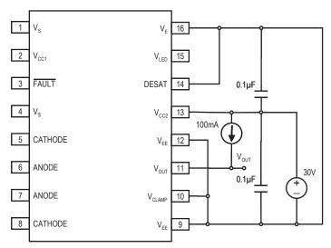
Figure 24. V<sub>OL</sub> Pulsed test circuit
