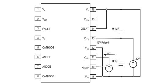
Figure 22. I<sub>OL</sub> Pulsed test circuit
