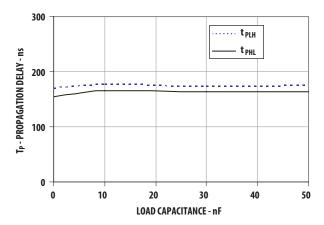
Figure 16. Propagation delay vs. load capacitance
