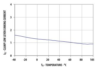
Figure 8. I<sub>CL</sub> vs. temperature
