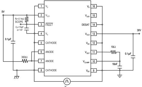
Figure 31. CMR Test circuit LED2 off
