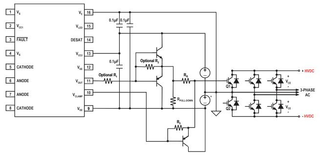
Figure 41. Large IGBT drive with negative gate drive, external booster. VCLAMP control secondary discharge path for higher power application.
