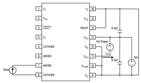
Figure 21. I<sub>OH</sub> Pulsed test circuit
