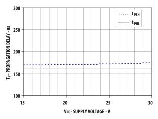
Figure 14. Propagation delay vs. supply voltage
