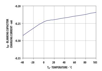
Figure 11. I<sub>CHG</sub> vs. temperature
