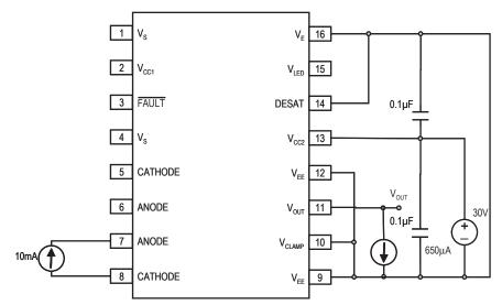
Figure 23.  $V_{OH}$  Pulsed test circuit
