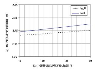
Figure 10.  $I_{\text{CC2}}$  vs.  $V_{\text{CC2}}$
