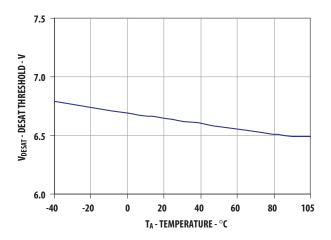
Figure 12. DESAT threshold vs. temperature
