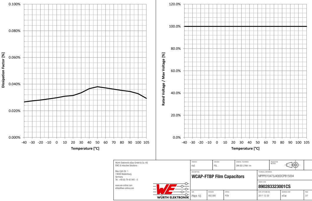
**Rated Voltage vs. Temperature:**
