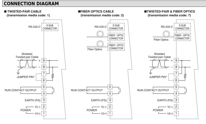
\*When the unit is located at the end of transmission line via twisted-pair cable (= no cross-wiring), short across the terminals 6 – 7 with the jumper pin (or wire) provided with the unit. Remove the jumper pin for all the unit not located at the end.
