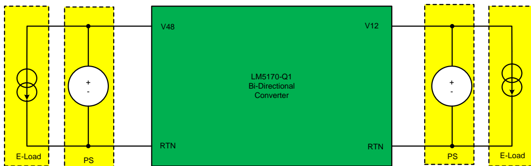
Figure 71. Emulated Dual Battery System With Bench Power Supplies and E-Loads
