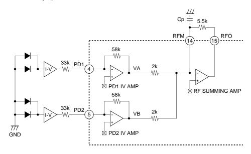
The frequency response of the RF output signal can be equalized by adding the capacitance (Cp) to RFI pin. The low frequency component of the RFO output voltage is as follows;
