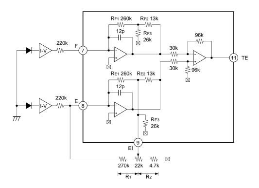
The balance adjustment is performed by varying the combined resistance value of the feedback resistors, which are T type-configured at the E I-V amplifier, by using the external resistance value of EI pin.
