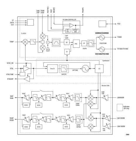
Figure 1. SKY74963 RF Transceiver Block Diagram
