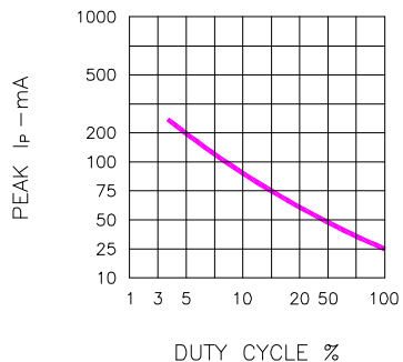
Fig.6 MAX PEAK CURRENT VS. DUTY CYCLE % (REFRESH RATE f=1 KHz)
