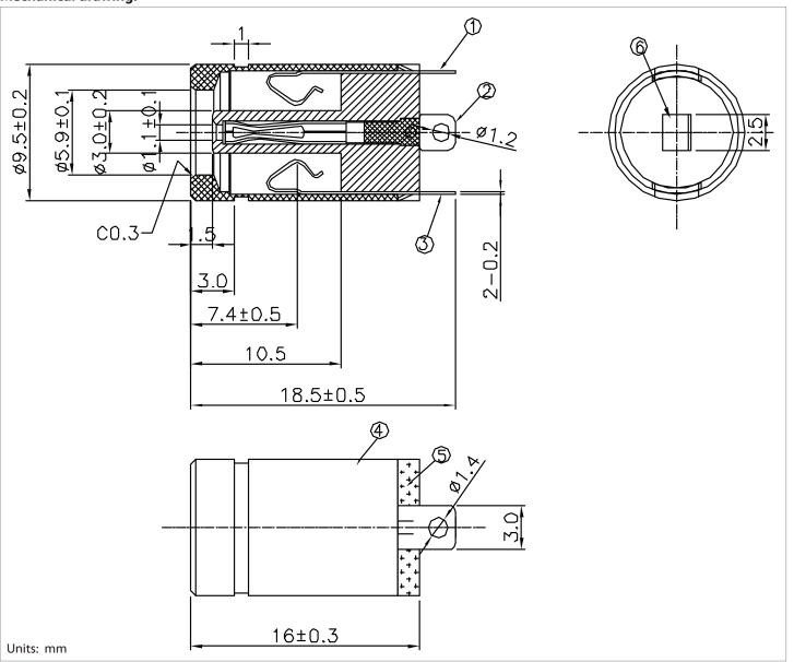
**tolerance** X: ±0.5 mm .X: ±0.3 mm .XX: ±0.05 mm applicable unless otherwise indicated in specification or on drawings
