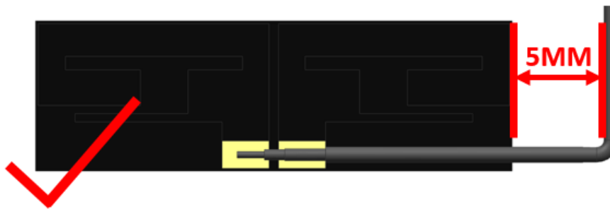
FIGURE 5.2.1 RECOMMENDED CABLE BENDING RANGE
