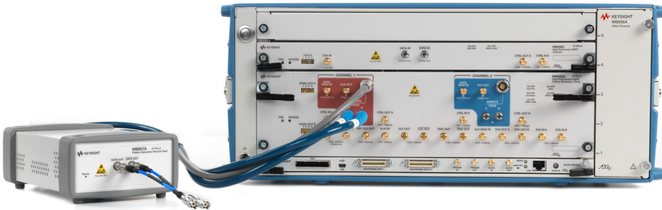
Figure 3. The remote head M8057A is required for each channel and is required for NRZ and PAM-4 signals. It contains an adjustable gain amplifier without re-timer. Users can select NRZ or PAM-4 coding and de-emphasis taps settings from the user interface with no need to reconnect cables. The cable between the remote head and the module is 0.85 m long. This allows positioning the remote head closely to the test board for the device under test.
