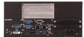
Expansion 4 slot (PCI-Express(x4)x1, PCIx3) type
