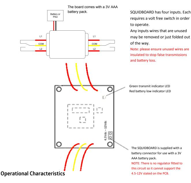
The SQUIDBOARD is very simple to connect and use. Simply wire a switch to any one or many of the inputs and send a signal.
